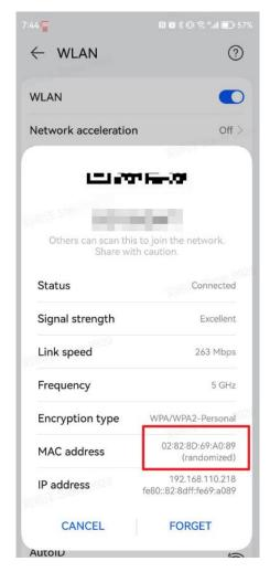
MAC addresses can be seen as IDs of devices which are unique. When making phones or other electronic devices, the manufacturer allocates a MAC address to each device. In the past, our phones have only the device MAC address. Therefore, when our phones try to connect to a network, our device MAC information will be obtained by others for them to track our phones and to obtain other information stored in our phones.
