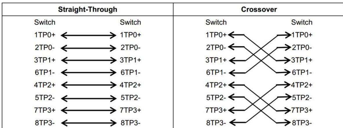
In addition to the above cables, the 100BASE-TX/10BASE-T can also use 100-ohm Category-3, 4, 5 cables for 10 Mbps, and 100-ohm Category-5 cables for 100 Mbps, both of which can be up to 100 m. Figure A-2 shows the pinouts of the 100BASE-TX/10BASE-T.
