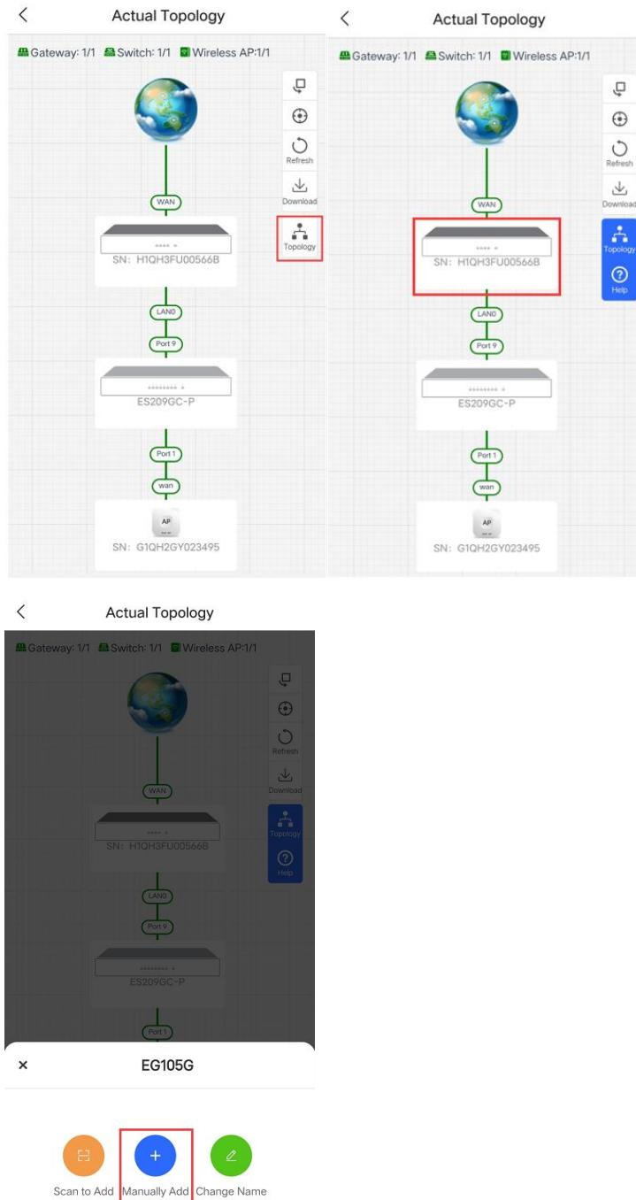
(3) Select the device model and its uplink port, and the device is added successfully.
