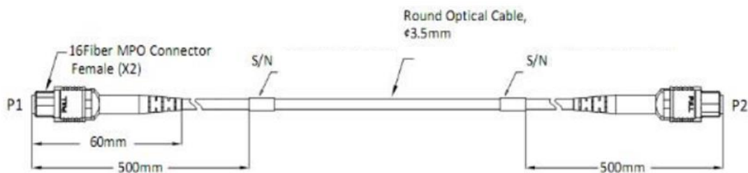
Figure 2-1 Structure of 16-Fiber MPO Fiber Jumpers
